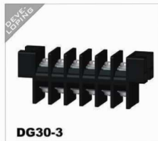
DG30-3 IEC 750V/101A 25.0mm 2 UL 600V/75A 10-2AWG
