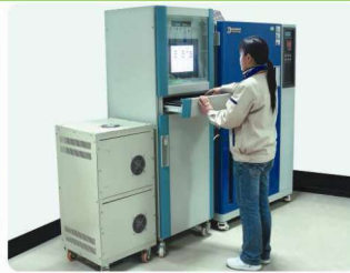
Heat cycling voltage drop test
