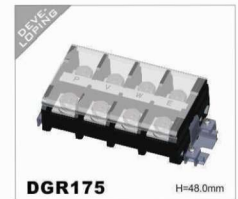
DGR175 H=48.0mm IEC 800V/175A 70.0mm 2 UL 600V/175A 20-2/0AWG
